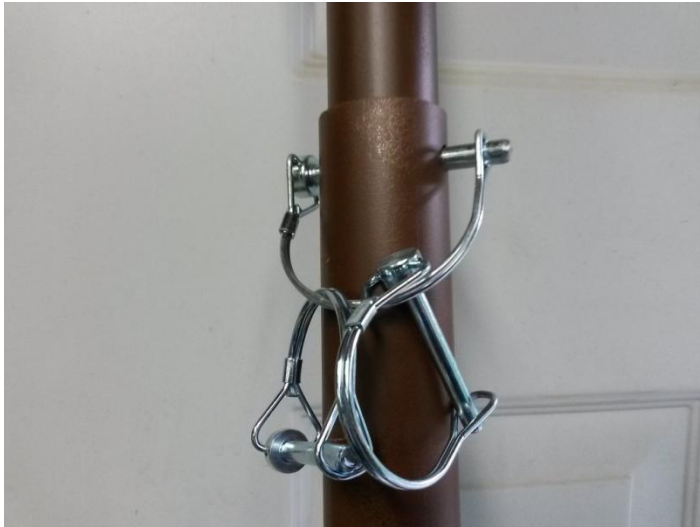
Pins used to secure sections
